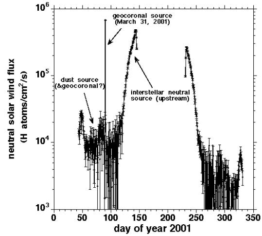
**FIGURE 2.** Neutral solar wind fluxes observed at IMAGE apogee during year 2001 illustrate the three major sources of neutral solar wind. Error bars indicate statistical uncertainties.
