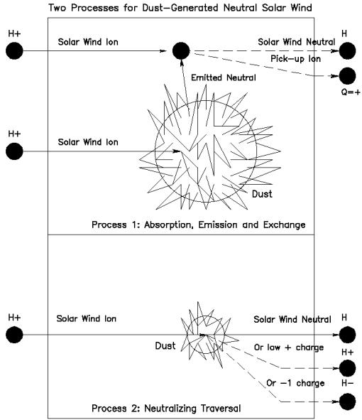
**FIGURE 1.** Dust creates solar wind neutrals either through a process of absorption, re-emission, and charge exchange or through a solar wind ion penetrating the dust grain and emerging on the other side in a neutral state.
